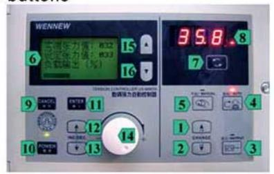
[1#], [2 #] key to duplex conversion key. Press 1 to # key, change to a working machineBit operation (the original is in the 2-position), press 2 # key, the machine change to 2 station (formerly at 1 station).
