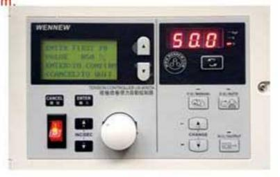
The display shows: Enter the sensitivity constant of integration and automatic operation of For, the lower the sensitivity, the larger the constant. Range 00-99, the general out Unwinding set before factory between 15-30, winding set at between 50-80, Press [Enter] key.
