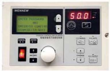
The display shows: Enter duplex conversion time in the range of 00-30 seconds, Rotating panel knob, as needed, enter the appropriate value, press [Enter] key to confirm.
