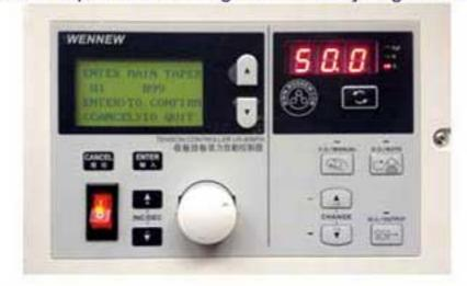
3. in the rolling work, please use this feature, enter the winding main taper value. Ranging from 01 to 99. The smaller the value, the slower the taper decreasing. Factory General Settings99.
