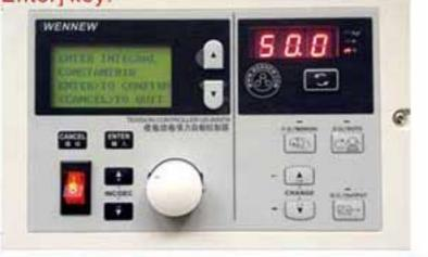
The display shows: Enter the brake voltage value% (terminal MI1, G closed effective) Generally used when unwinding work, using high-speed work.
