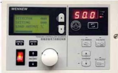
5. If you need to change the volume down, press 3 [output] key, the top this time Red light, the 6th screen displays "load off", the 8th-screen display "OFF", Load output temporarily closed. Change volume is completed, then the 3rd [output] key, the top of the red light is off, all Display restitution, loads opened a new round of work is resumed.
