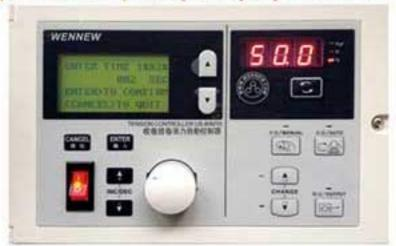
Screen: Please enter F0 is the initial value of the load voltage percent(Each reset or duplex convert that value) in the range of F00-F99,Rotating panel knob and press [Enter] key to confirm.
