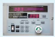
3. Press ENTER key until screen shows T01 (It is the time for a two part alternation, set up the same way as the set up for F). For example, rotate the digital set trimmer and adjust the initial value of time to current time 0-30 secretary.
