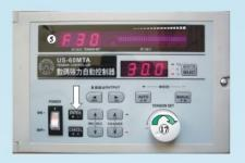
5. If new material roll change is needed, press the load output OFF key to stop load output.
