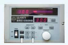
8. Please turn on #4 switch. This means that the controller works directly from manual to auto, the outer counting ring (need to be removed) is invalid under the auto state.
