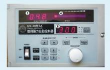
7. Adjusting the #2 sensor-turn on the #1 sensor switch before turning off the #2 sensor switch. Then rotate #2 micro adjustment set trimmer to desired value (value will increase when rotated clockwise, and decrease when rotate to anticlockwise to lowest value 00.0).
