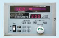
3. Press the AUTOMATIC key. The green and red light above the key will blink alternately for 5 seconds. If the red light is lit and the green light out, then auto status is working.
