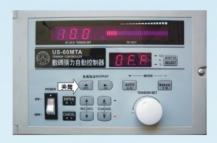
6. After changing the material roll, press the load output ON key to recover the load output.
