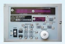
1-- Power switch. "On" is turn on the machine, "OFF" is turn off the machine.
