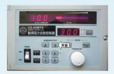
7. Press #1 or #2 two-work parts key and the CANCLE key, the #8 LED shows the initial value of voltage percent, it is ready to start the new work. (If no function of two-work parts, please press the CANCLE key)
