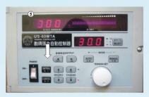
2x Rotate the auto digital set trimmer, put in password "07".
