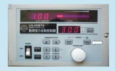
2. Rotate the digital set trimmer, adjust the manual tension to an appropriate value (example-30.0). The max value is 50.0, or 100% load. The controller can't enter the automatic status until it obtains the value necessary for maintaining normal state tension (example-10 kgf).
