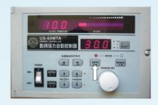
4. This machine is now working under the normal conditions. #5 LED will show the initial tension set value, screen #6 will show present tension value and #8 LED will show the voltage percent value.
