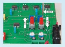
6. The result of #1 sensor adjustment is only acceptable if the #5 LED presents a number in the range of 01.0 to 07.0 and screen #6 shows 2 or 3 bars.
