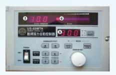
5. If the tension is not appropriate, then micro adjust the #17 set trimmer to obtain a valid tension set value for #5 LED.
