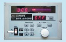
5. Adjusting the #1 sensor- turn on the #2 sensor switch before turning off the 1# sensor switch. Then rotate the #1 micro adjustment set trimmer to desired value (value will increase when rotated clockwise, and will decrease when rotated anticlockwise to lowest value 00.0).
